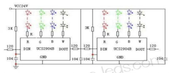
During 24V power supply, it is recommended that a 120 resistance be connected in series at the signal input and output ends of the IC to prevent damage to the IC input and output ends in case of live plugging or power supply and signal wires being wrongly connected. In addition to the parallel connection of a 104 capacitor between VDD and GND of IC, a 104 capacitor must also be connected between VCC and GND to reduce ground wire surge interference
