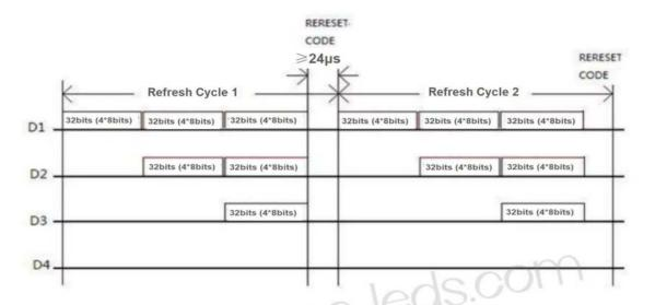
Note: D1 is the data sent by MCU, and D2, D3 and D4 are the data automatically reshaped and forwarded by cascade circuit.
