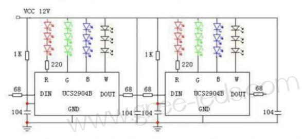
During 12V power supply, it is recommended that a 68-120 resistor be connected in series at the signal input and output ends of the IC to prevent damage to the IC input and output ends in case of live plugging or reverse connection of power and signal wires. In addition to the parallel connection of a 104 capacitor between VDD and GND of IC, a 104 capacitor must also be connected between VCC and GND to reduce ground wire surge interference
