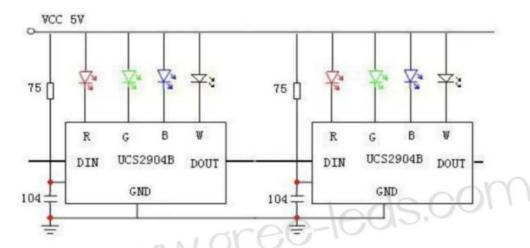
The constant current mode can achieve the ideal effect of keeping the brightness and color temperature unchanged while the voltage drops continuously.
