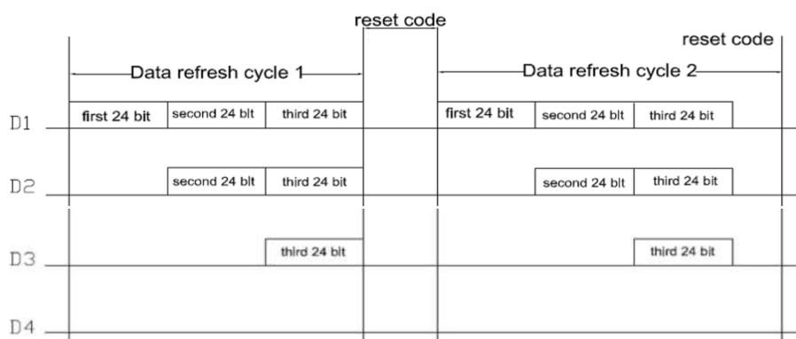
Note: D1 is the data sent by the MCU, and D2, D3, and D4 are the data that the cascade circuit automatically reshapes and forwards.
