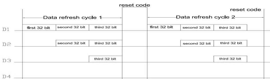
Note: the D1 sends data for MCU, D2, D3, D4 for data forwarding automatic shaping cascade circuit.
