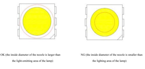
Pressing the colloid surface will affect the reliability of LED because the LED is advanced silicone-gel.And therefore precautions should be taken to avoid the strong pressure on the component. It's proper to make the LED be used in safe condition when using a suction nozzle. Silicon packing with soft and elastic, it greatly reduces thermal stresses and unable to bear external mechanical forces. Therefore, preventive measures should be taken in process of manually handling.
