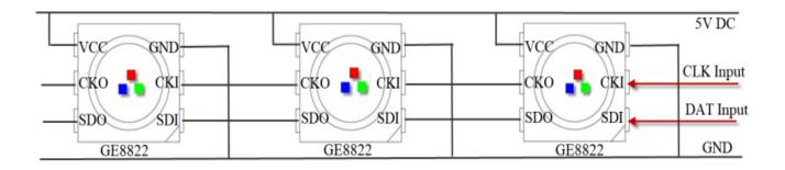
In the practical application circuit, the signal input and output pins of the IC signal input and output pins should be connected to the signal input and output terminals. In addition, in order to make the IC chip is more stable, even the capacitance between beads is essential back;
